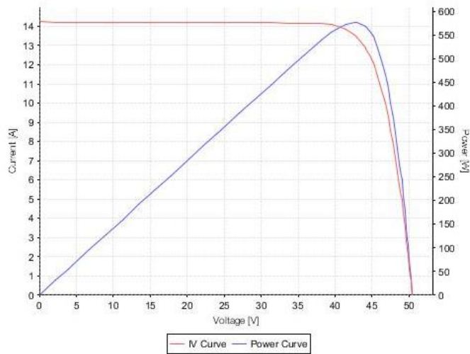
Fig. 6 IV curve of module No.2 Serial number: ASA22190800173
