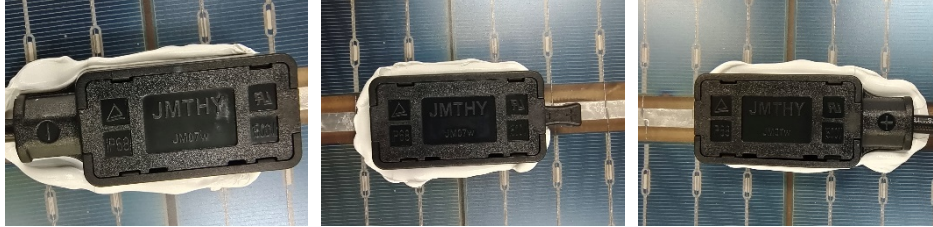
Fig. 3: View of junction box of module type ERA Pro-72HCB575M
